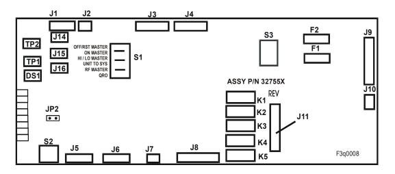
Figure 10. Location of Programming Switch S1 on PWB
